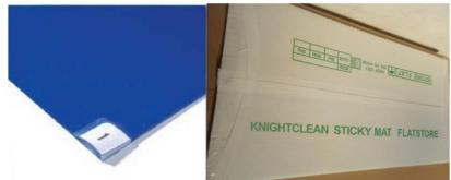
A sticky mat is a mat with an adhesive surface that is placed at the entrances to certain workplaces to remove contaminants from the bottoms of footwear and wheeled carts. Sticky mats are typically used in cleanrooms. Their purpose is to prevent dust and contaminants from entering the area. Sticky mats are made of a stack of adhesive plastic film layers that are periodically peeled off and discarded.
